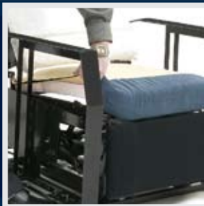
Attach hook & loop strip to seat box & pull back tight
