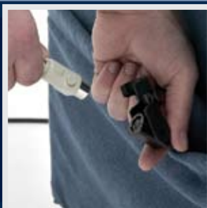
Plug hand controller into quick release cable
