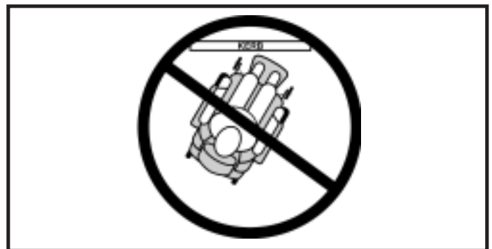
Figure 3. Incorrect Kerb Approach
