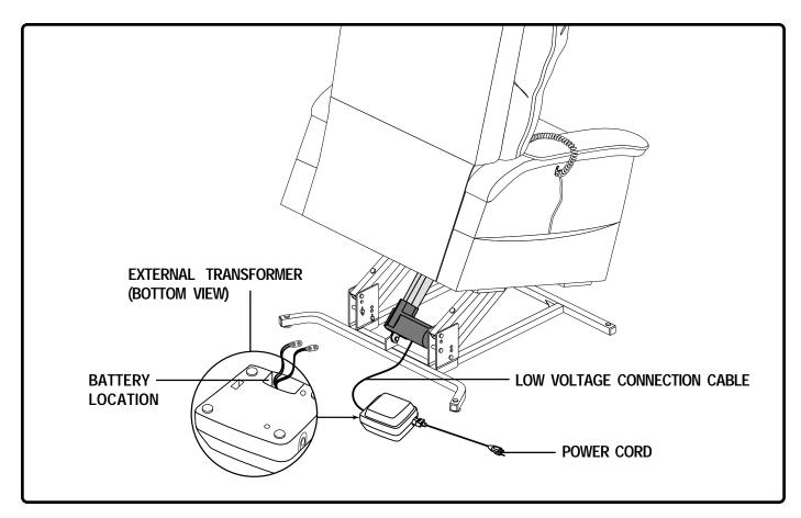
Figure 4.3 Heat and Massage Lift Chair Battery Location (Including 555 model)
