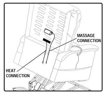
4.1.4. If your chair is equipped with heat and/or massage options, connect the quick-release connections on the chair-back at this time.
