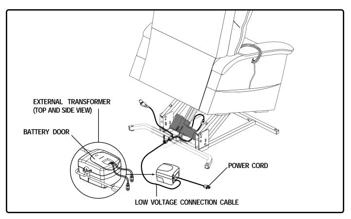
Figure 4.2 Standard Lift Chair Battery Location
