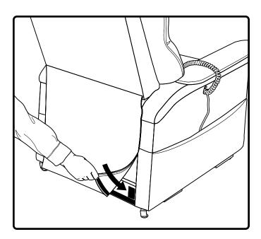
4.1.5. Attach the chair-back to the hook and loop flaps on the bottom of the chair base.
