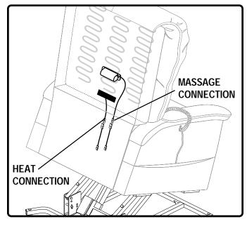
4.4.2. If your lift chair is equipped with heat and/or massage options, locate the quick-release connections, grip the plastic ends, and pull the connections apart. Avoid pulling on the wires when making the disconnection.
