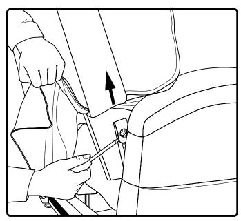
4.4.3. Using a large flat-head screwdriver, lift the left and right locking clips on the chair-back one side at a time to raise the back from the connections on the chair base. As you lift each locking clip, pull up on the chair-back to lift that side over the lock.
