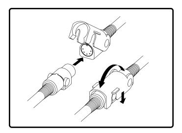
Figure 3.5 Quick-Release Connector
