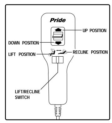
Figure 5.3 Infinite Series Hand Control
