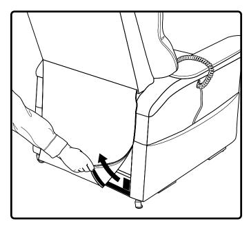
4.4.1. Remove the bottom of the back fabric from the hook and loop flaps on the chair base.
