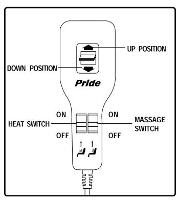
Figure 5.2 Heat and Massage Hand Control
