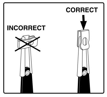
4.1.1. Remove the packaging from the back portion of the chair and check that the locking clip is in the vertical position. Reposition if necessary.
