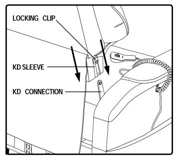
4.1.2. Slide the left and right KD sleeves of the chairback onto the KD connections on the arms and seat of the chair.
