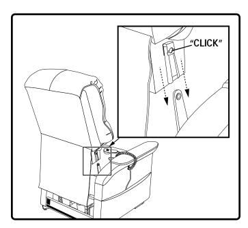
4.1.3. Push firmly on the top of the chair-back to lock into position. Listen for a click on each side to ensure the chair-back is locked in properly.
