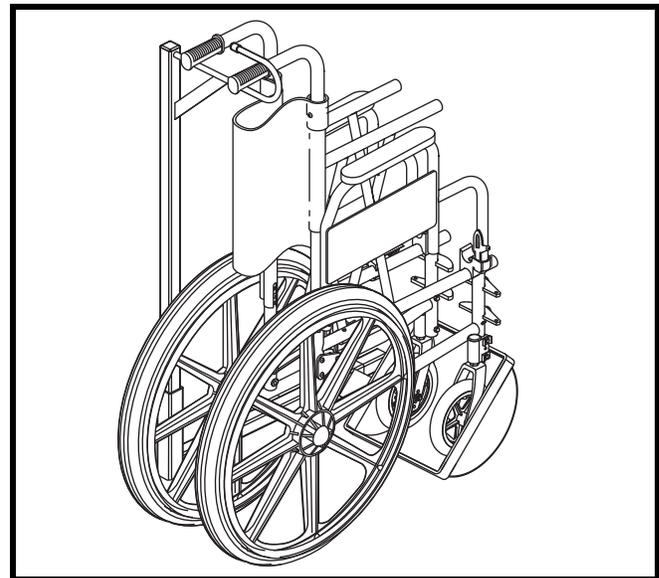
6. Lift the folded wheelchair and place the front caster wheels in the front caster bracket. Secure the wheelchair handles over the vertical hook post.
