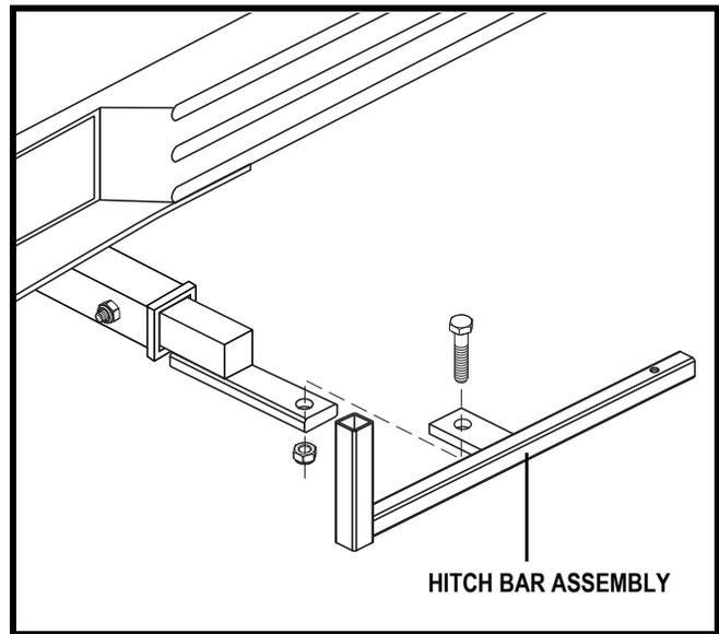
1. Install the hitch tube to the vehicle hitch tube receiver. Insert the hitch bolt from the passenger's side through to the driver's side of the hitch.
