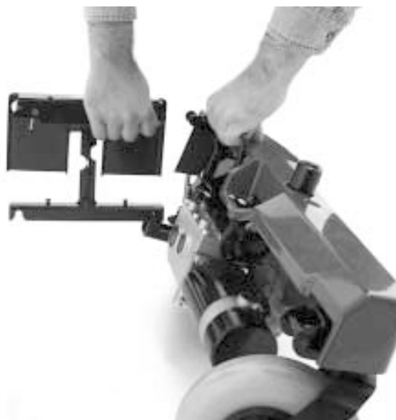
Figure 19. Connecting Front Frame Assembly
