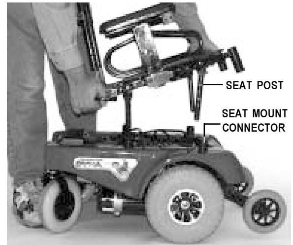
Figure 13. Removing the Versa Seat
