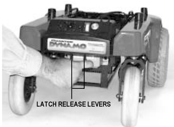
Figure 16. Removing Battery Well Frame
