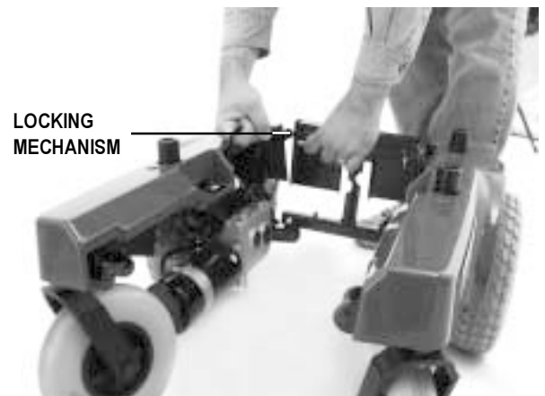
Figure 20. Fitting the Frames
