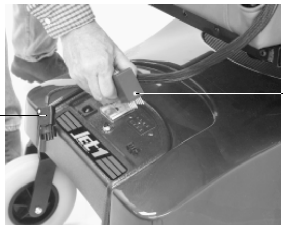
Figure 10A. Controller Harnesses
