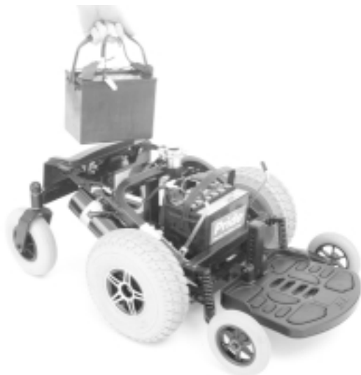
Figure 7. Removing the Batteries from Your Jet 3
