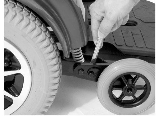
Figure 29. Anti-Tip Wheel Adjustment
