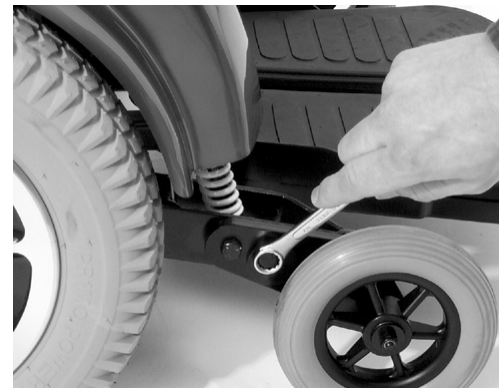
Figure 30. Anti-Tip Wheel Adjustment
