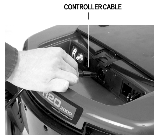
Figure 11. Controller Cable Connection
