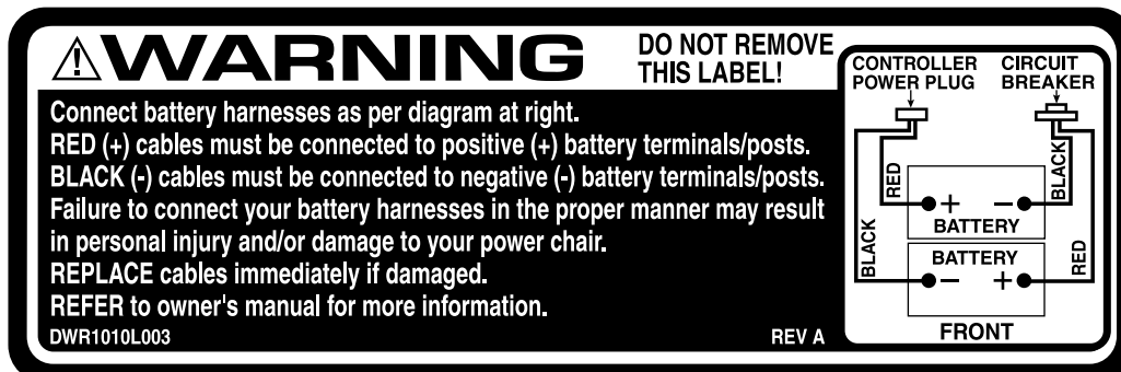
Figure 24. 1400 Series Battery Wiring Diagram Label
