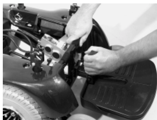
Figure 25. Installation du Repose-pied
