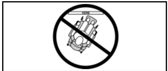
Figure 3. Incorrect Kerb Approach
