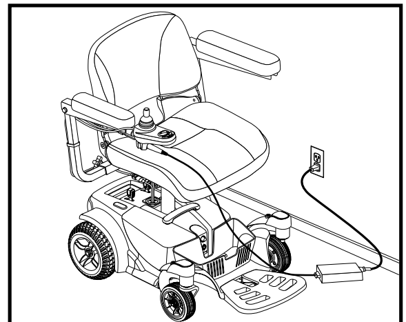
Figure 24. Battery Charging through the Controller
