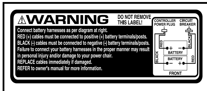
Figure 28. Battery Wiring Diagram Label
