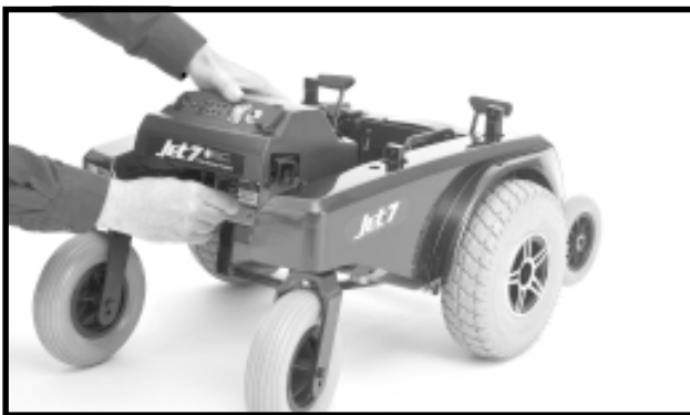
Figure 17. Removing Battery Well Frame
