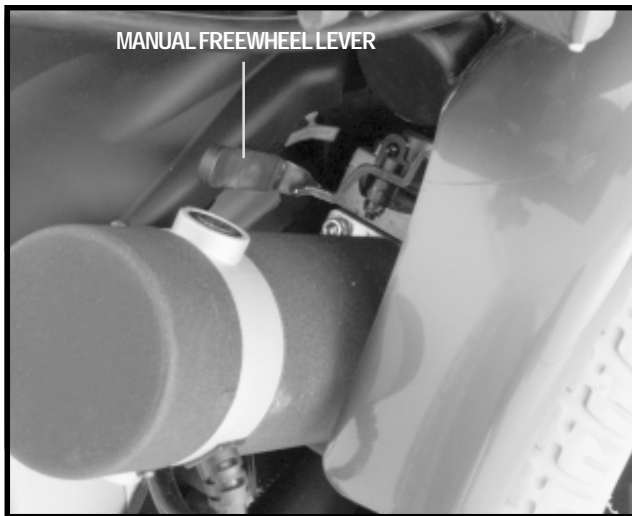
Figure 7. Freewheel Mode (Drive Disengaged)
