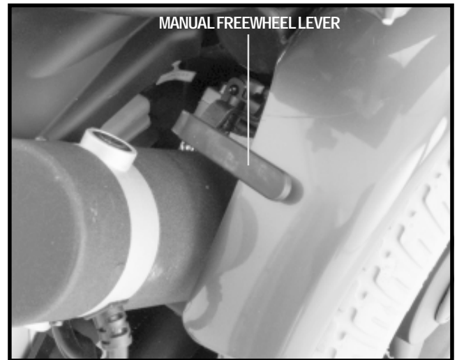
Figure 8. Drive Mode (Drive Engaged)
