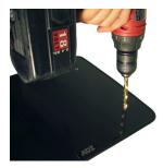
9. Drill four 3/16in. holes where the seat base is marked.
