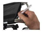
Prior to removing OEM seat sling, mark left and right chair frame at the front edge of the OEM seat sling.
