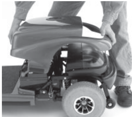
FIGURE 19. REAR SHROUD REMOVAL
