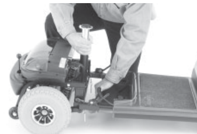
FIGURE 25. SEPARATING THE FRAME SECTIONS
