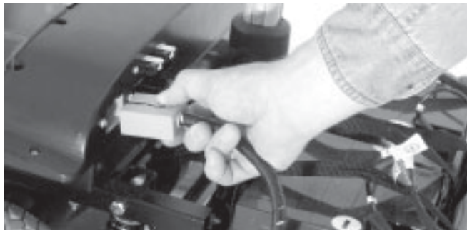
FIGURE 21. DISCONNECTING THE FRONT-TO-REAR HARNESS
