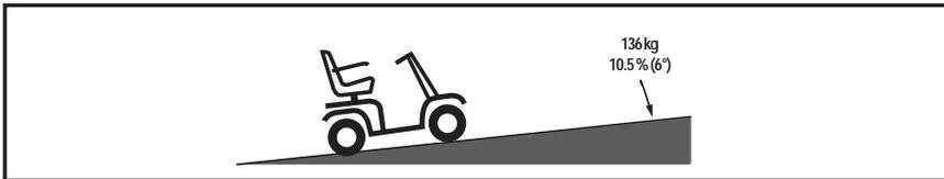
Figure 1. Maximum Recommended Incline Angle
