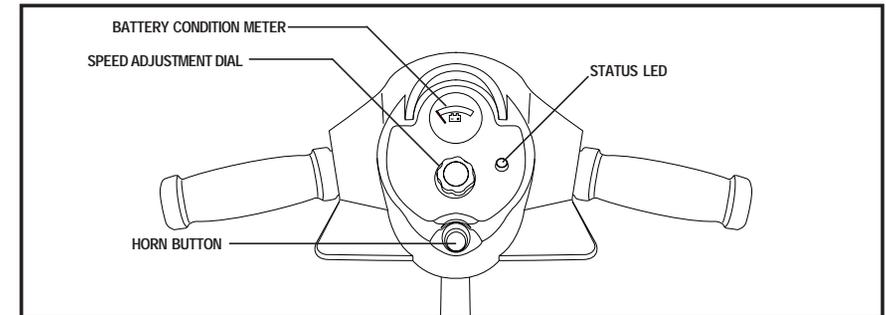
Figure 5. Upper Tiller Console Components
