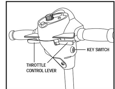
Figure 5A. Lower Tiller Console Components
