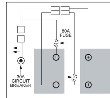
Figure 8A. Battery Wiring Diagram
