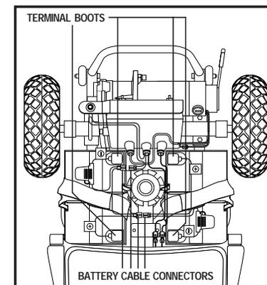
Figure 8. Battery Connections
