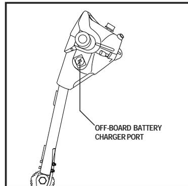
Figure 5B. Off-board Battery Charger Port
