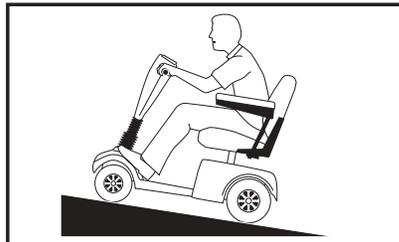
Figure 2A. Increased Stability Driving Position
