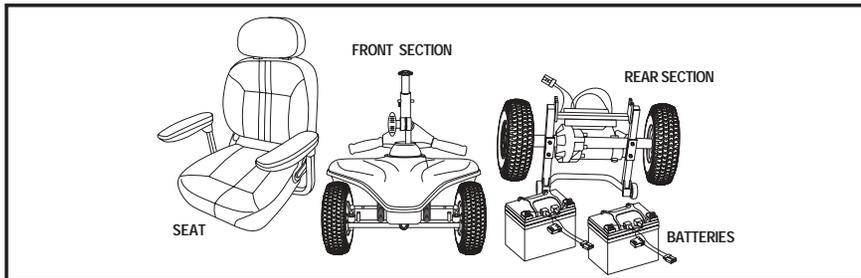
Figure 13. Scooter Components
