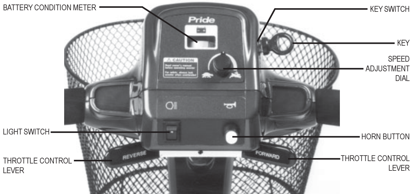
FIGURE 7. CONTROL CONSOLE ASSEMBLY
