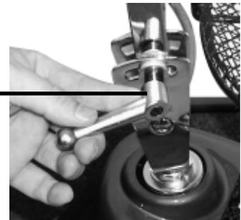
**Figure 8b. Reposition Tiller Adjustment**
