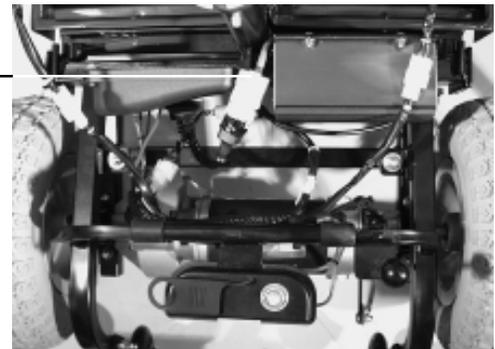
Figure 14. Front-to-Rear Connector
