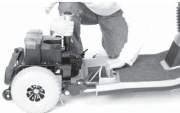
FIGURE 25. SEPARATION DES SECTIONS AVANT ET ARRIÈRE
