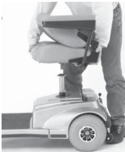
FIGURE 18. ENLÈVEMENT DU SIÈGE
