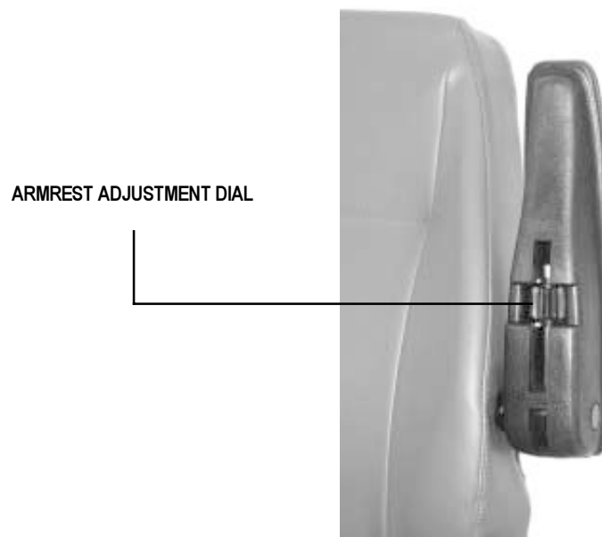
Figure 20. Armrest Angle Adjustment
