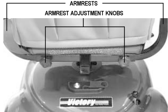
Figure 19. Armrest Width Adjustment
