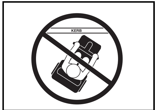
Figure 3A. Incorrect Kerb Approach
