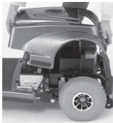
FIGURE 19. REMOVING THE SHROUD
