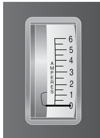
Figure 10. Ammeter Indicates Batteries Are Fully Charged
