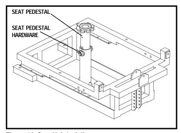
Figure 10. Seat Height Adjustment
