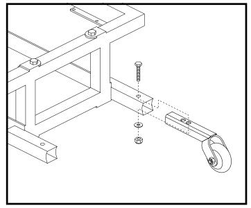
Figure 18. Anti-Tip Wheel Assembly
