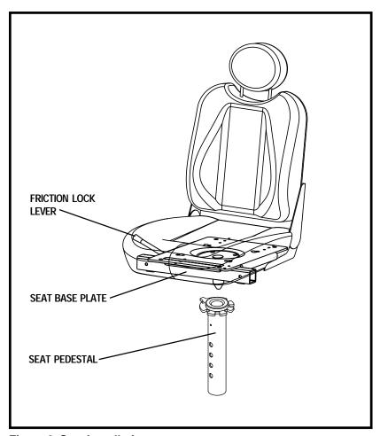
Figure 9. Seat Installation
