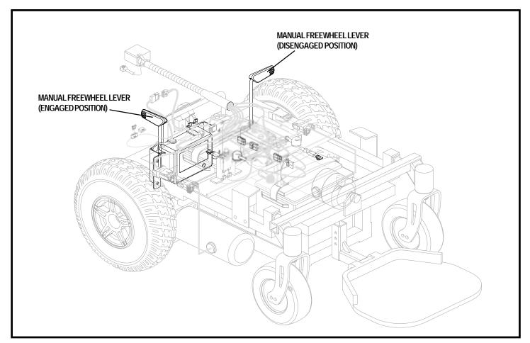
Figure 8. Manual Freewheel Lever Positions
