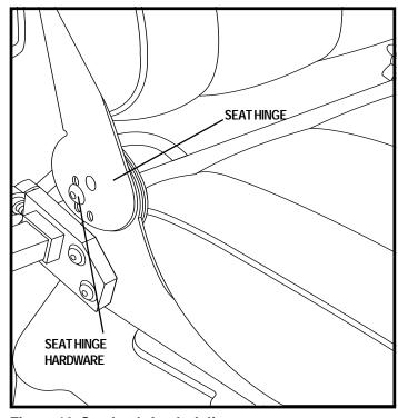
Figure 12. Seatback Angle Adjustment
