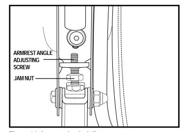
Figure 14. Armrest Angle Adjustment
