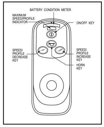
Figure 21. VSI Controller Keypad
