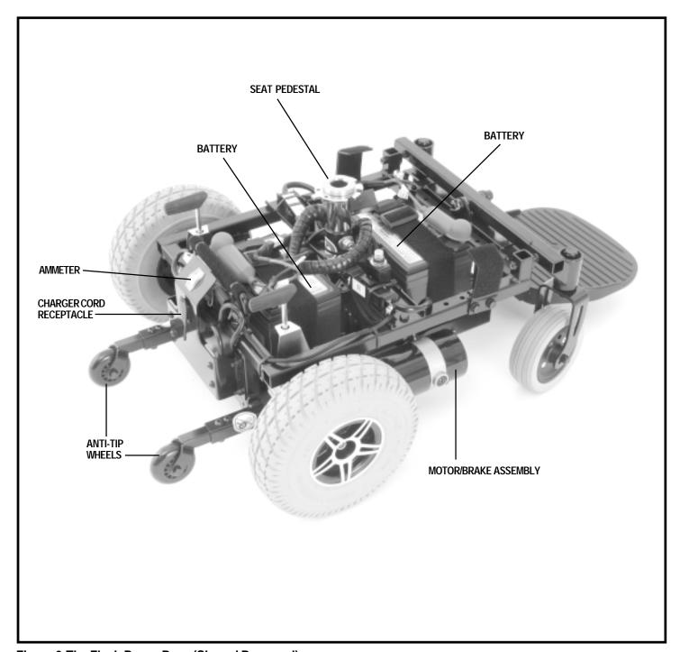
Figure 6. The Flash Power Base (Shroud Removed)
