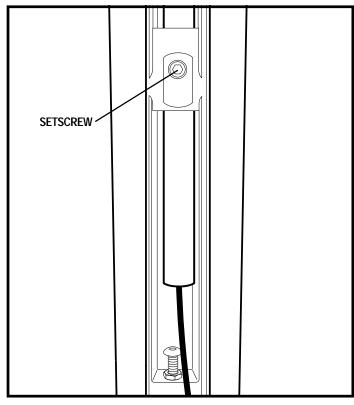
Figure 16. Underside of Armrest
