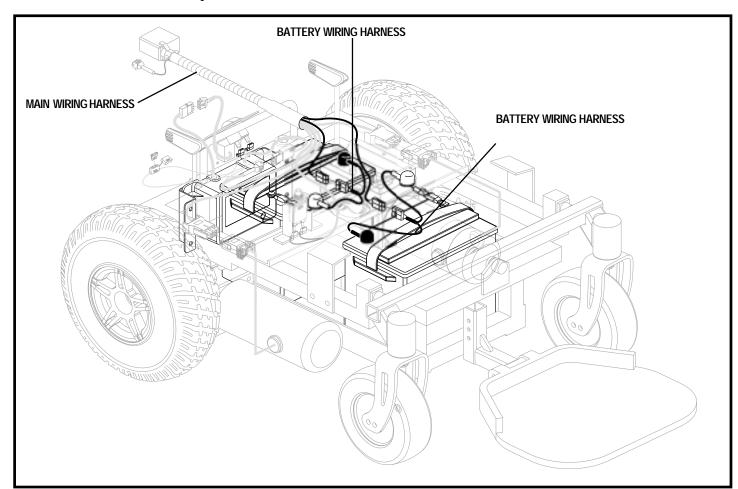
Figure 23. Flash Battery Connections
