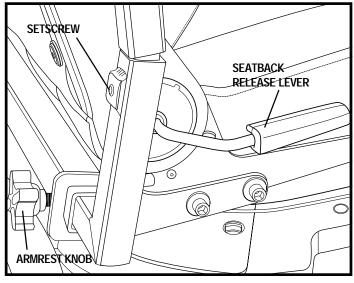
Figure 13. Seat and Armrest Adjustments
