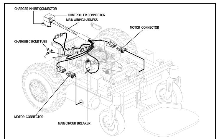
Figure 7. Flash Electrical Components
