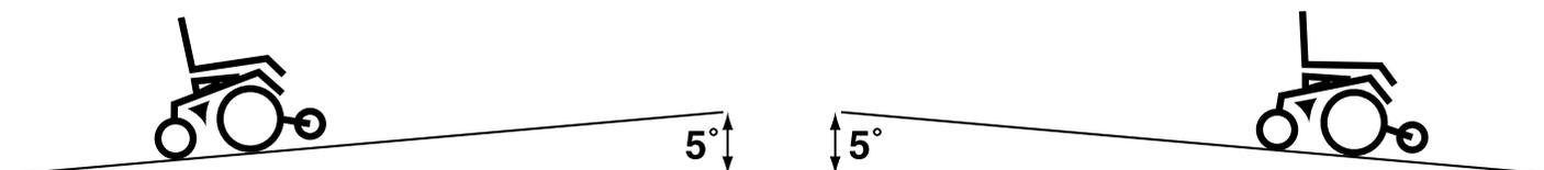
Figure 1. Maximum Safe Angle (Ascending and Descending)
