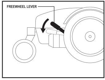
Figure 5. Freewheel Mode (Drive Disengaged)
