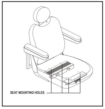
Figure 17. Seat Position Adjustment
