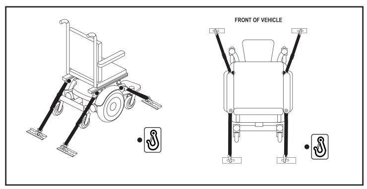
Figure 14. Unoccupied Transit System Securement Points
