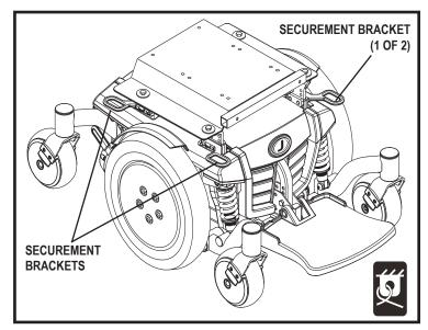
Figure 13. Transit System Securement Brackets-UK Occupied Transit
