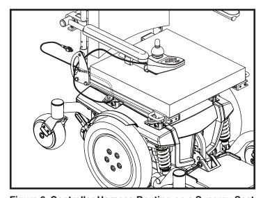
Figure 9. Controller Harness Routing on a Synergy Seat
