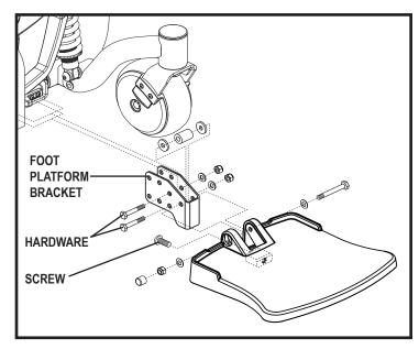
Figure 20. Foot Platform Adjustment
