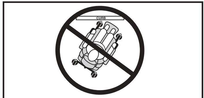
Figure 3. Incorrect Curb Approach
