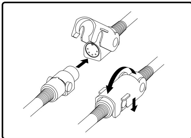
Figure 3.5 Quick-Release Connector
