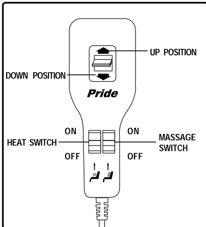
Figure 5.2 Heat and Massage Hand Control
