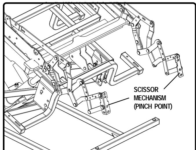
**Figure 3.3 Scissor Mechanism**
