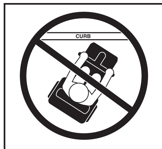
Figure 7. Incorrect Curb Approach
