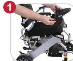
1 Switch off and remove joystick
