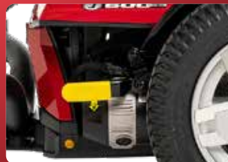
Easy-access free-wheel lever
