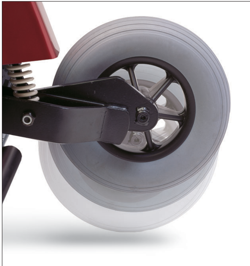
Front anti-tip wheel shown in lowered, normal and raised positions
