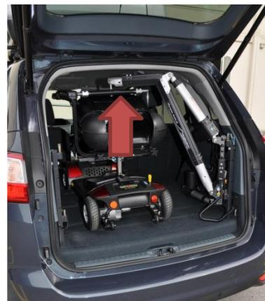
6. While retaining the handset move clear of the Hoist and its path of operation
