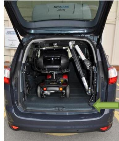
15. Press and hold the down button until the scooter/chair is firmly placed on to the vehicle floor.
