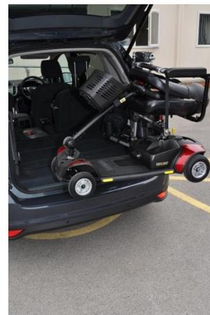
12. Press and hold up button to raise the scooter/chair up to the upmost position then release button steady the scooter during operation and ensure it does no contact the vehicle.
