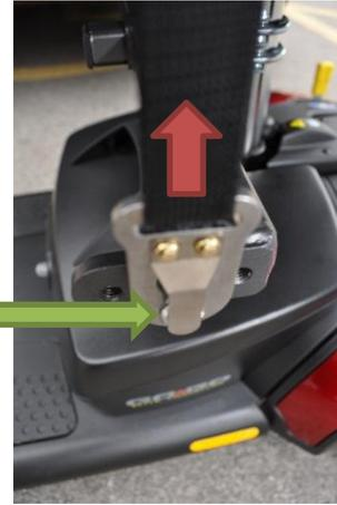
11. Engage the keyhole plates securely to the lifting bracket. (This bracket will vary depending on what is being lifted)
