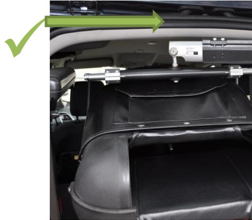
8. Press and hold the left or right button (depending on side of installation) to move the hoist outwards, steady the scooter/chair during operation and guide it smoothly out of the vehicle.
