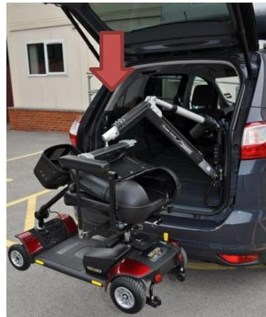
10. Press and hold the down button until the scooter/chair is grounded and there is some slack on the lifting straps.
