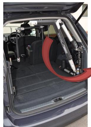
5. While retaining the handset move clear of the Hoist and its path of operation
