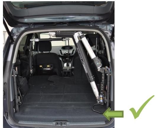
14. Return the handset back into its docked position – ensure the cable is clear of trapping hazards.
