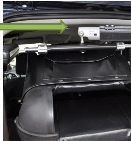
13. Press and hold the left or right button (depending on side of installation) to move the hoist inwards - steady the scooter/chair during operation and guide it smoothly towards the vehicle.
