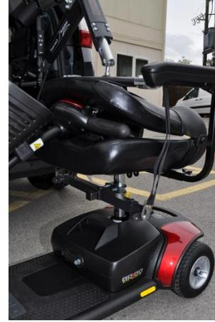
7. Release button when the boom is at its outmost position.
