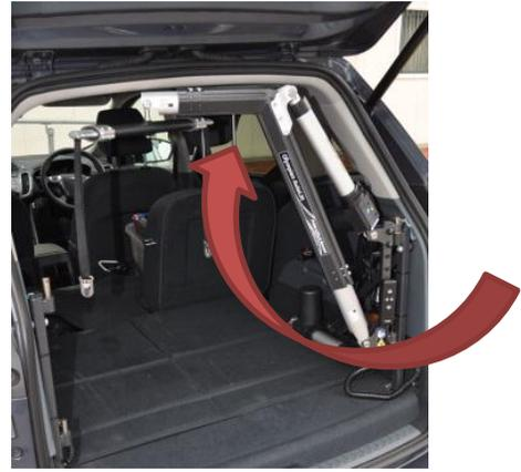
12. Ensure the scooter/chair is free from Hoist. Press the up button to raise the boom fully upwards
