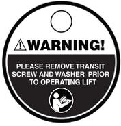
Remove transit screw and washer prior to operating the lift for the first time.
