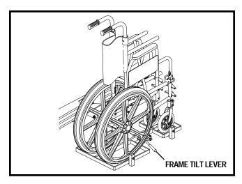
6. Squeeze the frame tilt lever and rotate the frame to the horizontal position.
