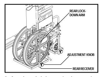
8. Insert the rear lock-down arm into the rear receiver. Position the lock-down arm firmly over the drive wheels and secure with the adjustment knob.
