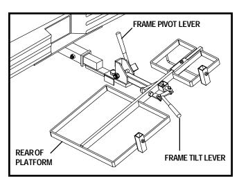
4. Squeeze the frame tilt lever and push down on the rear of the platform to tilt the platform to the ground.
