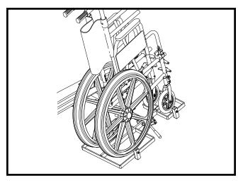
Position the folded wheelchair onto the carrier platform and engage the wheelchair park brakes.
