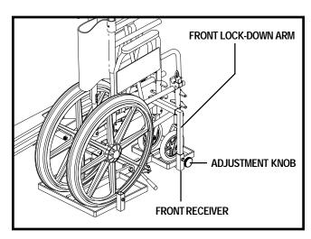
7. Insert the front lock-down arm into the front receiver. Position the lock-down arm firmly over the front caster wheel frame and secure with the adjustment knob.
