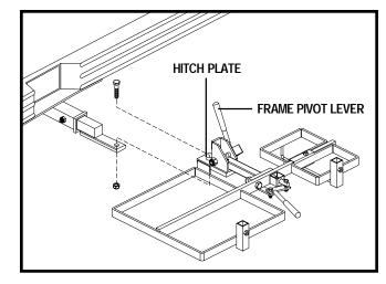
1. Install the hitch tube into the vehicle hitch tube receiver. Insert the bolt from the passenger's side through to the driver's side of the hitch.
