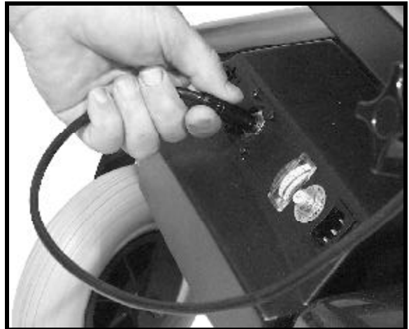
Figure 14. Disconnect the Controller Connector
