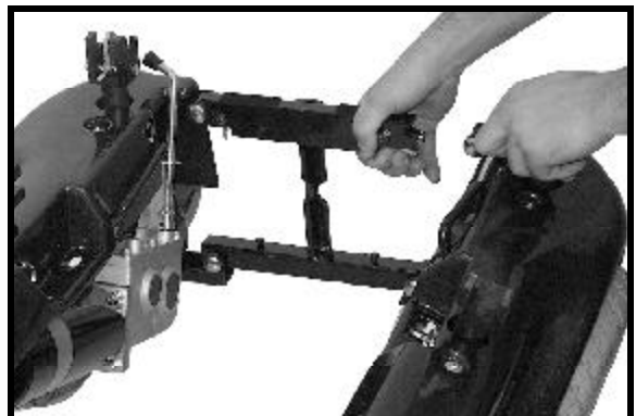
Figure 18. Side Frame Removal
