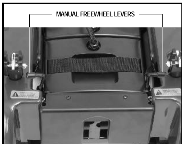
Figure 8. Drive Motor Disengaged
