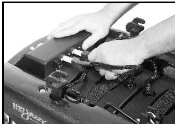
Figure 40. Disconnecting Battery Connectors
