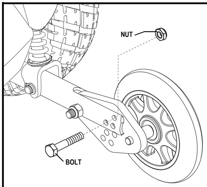
Figure 19. Anti-Tip Wheel Adjustment
