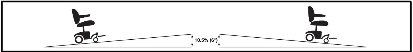
Figure 1. Maximum Recommended Safe Slope (Ascending and Descending)
