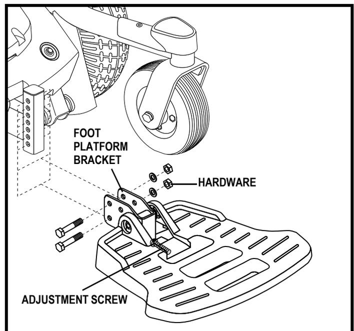
Figure 16. Select 6 Foot Platform Adjustment
