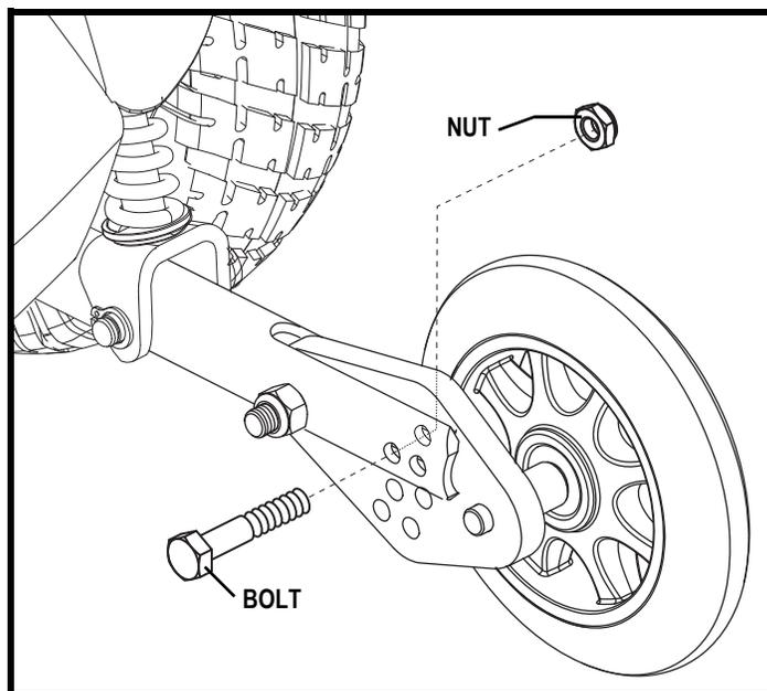
Figure 19. Anti-Tip Wheel Adjustment
