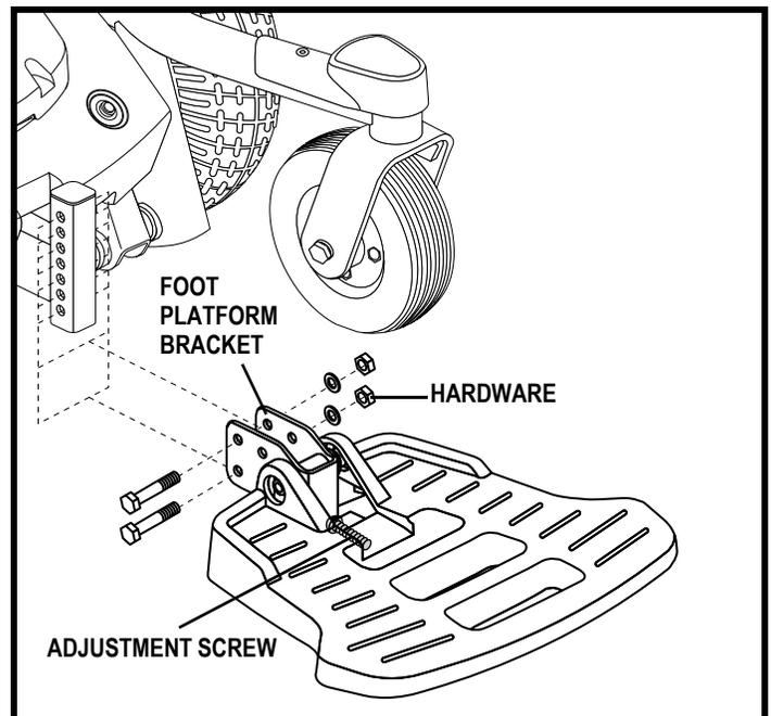
Figure 16. Select 6 Foot Platform Adjustment
