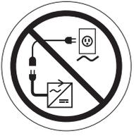
**Do not connect an extension lead to the AC/DC converter or the battery charger.**
