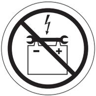
**Keep tools and other metal objects away from battery terminals. Contact with tools can cause electrical shock.**
