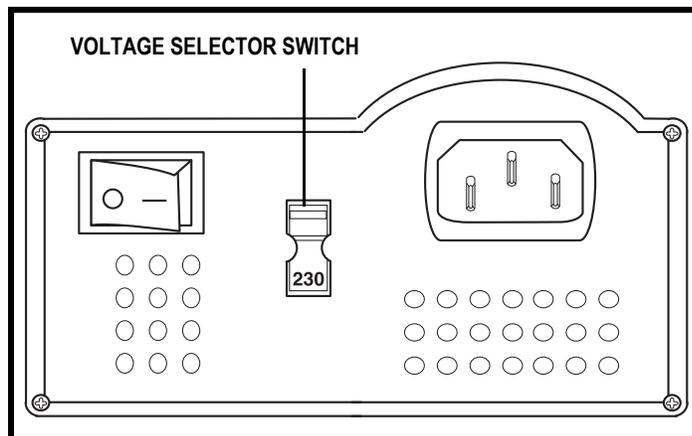
Figure 21. Manual Voltage Switch Off-board Charger
