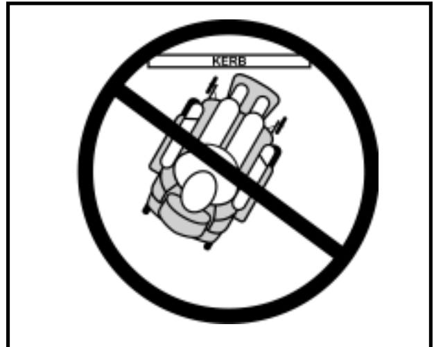
Figure 3. Incorrect Kerb Approach
