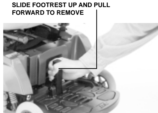
Figure 18. Removing the Footrest
