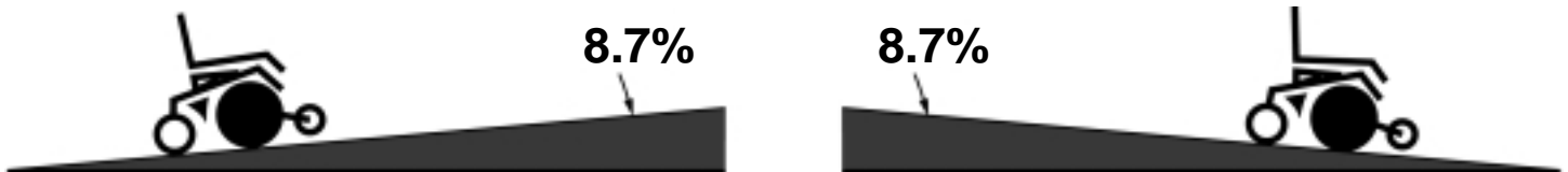
Figure 3. Maximum Recommended Safe Slope
