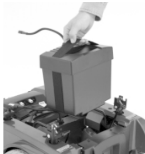
Figure 19. Removing Battery Boxes
