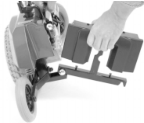
Figure 23. Connecting Front Frame Assembly
