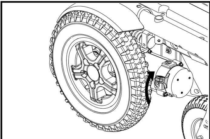
**Figure 9. Drive Mode (Drive Engaged) - Hammer and H2 Motors**
