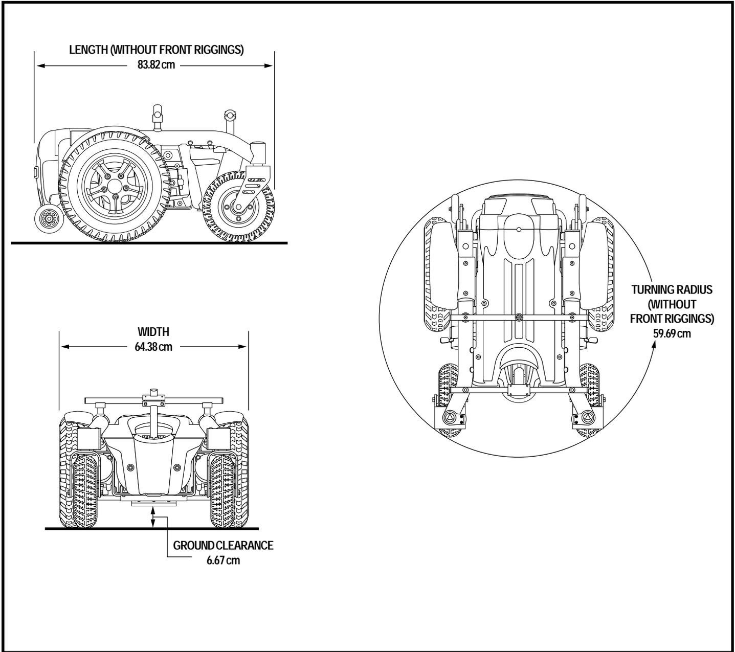
Figure 25. Quantum R-4000 Series Dimensions and Ground Clearance
