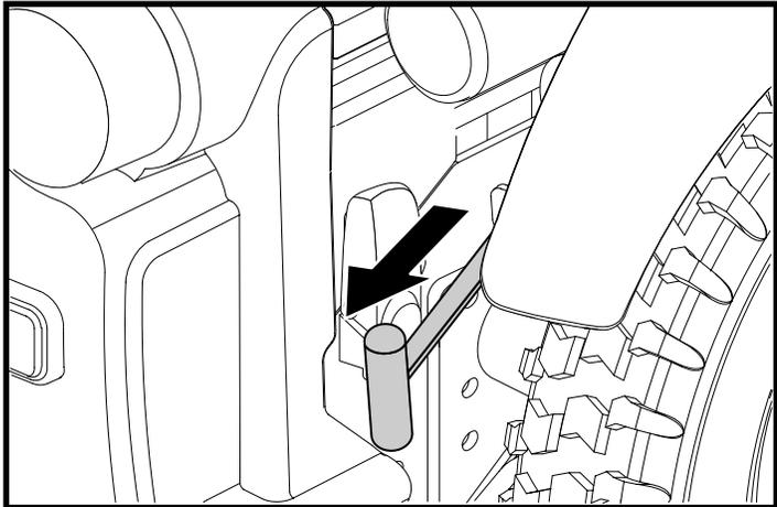
**Figure 10. Freewheel Mode (Drive Disengaged) - Glide Motor**
