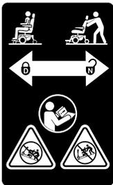
Left freewheel lever operation. Place unit on level ground and stand to one side when changing from drive mode to freewheel mode or freewheel mode to drive mode.
