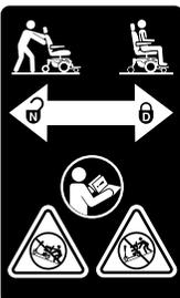
Right freewheel lever operation. Place unit on level ground and stand to one side when changing from drive mode to freewheel mode or freewheel mode to drive mode.
