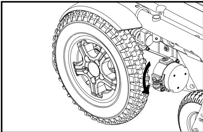
**Figure 8. Freewheel Mode (Drive Disengaged) - Hammer and H2 Motors**
