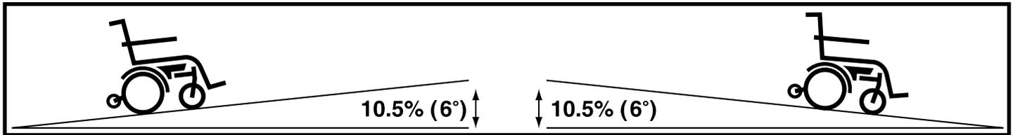
Figure 1. Maximum Safe Slope (Ascending and Descending)
