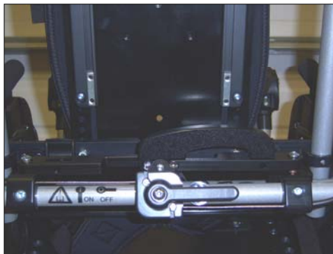
Figure 17: Hip Angle Adjustment Lever in locked position
