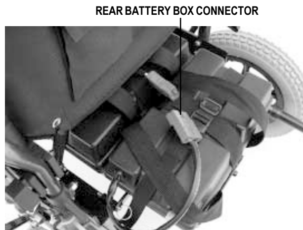
Figure 16. Rear Battery Box
