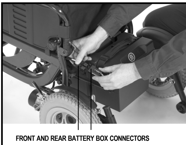
Figure 8. Front and Rear Battery Box Connection
