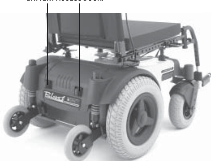
Fig. 5. Battery Access Door in Up Position
