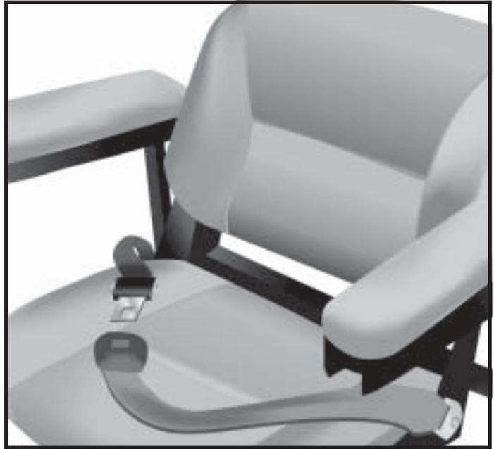
Figure 23. Positioning Belt
