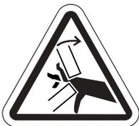
Pinch/Crush points created during assembly.
