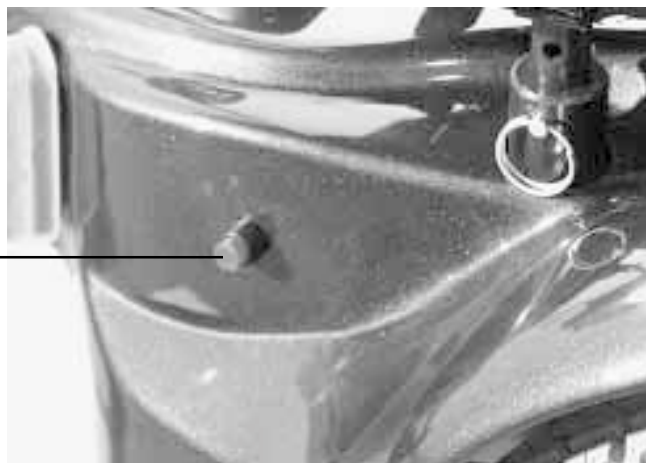
Figure 49. Standard Lighting Package Light Switch
