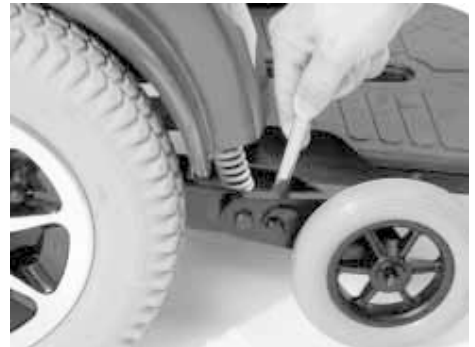
Figure 29. Anti-Tip Wheel Adjustment
