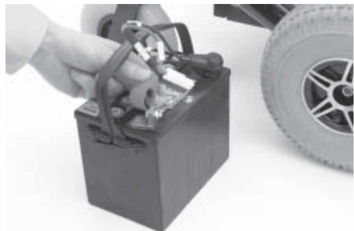
Figure 7. Connecting Wires to the Battery Terminals
