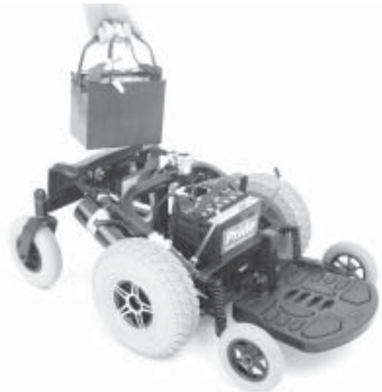
Figure 6. Removing the Batteries from Your Jet 3
