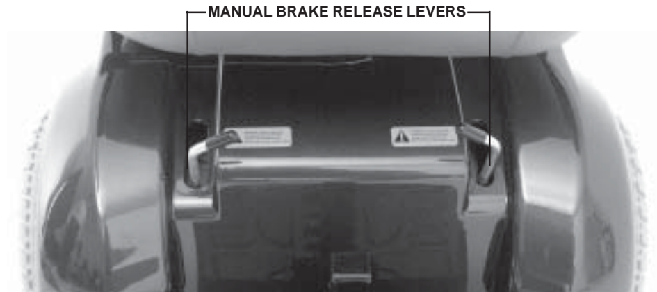
Figure 9. Drive Motors Disengaged (Freewheel Mode)
