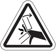
**Pinch/Crush points created during assembly.**
