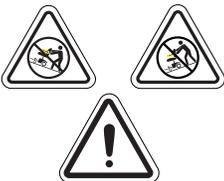
**WARNING! Do not use the power chair while the drive motors are disengaged! Do not disengage the drive motors when the power chair is on an incline or decline, as the unit could roll on its own. Only engage the freewheel mode when on a level surface.**
