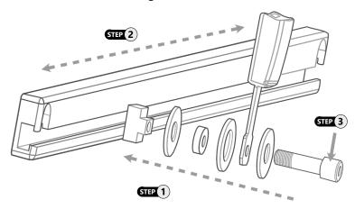
**Step 1:** Take the seat belt receptacle and one of the included hardware packages. Remove the M8 screw from the package and thread the other components on it in the following order: 5/16" washer, seat belt receptacle, M12 washer, spacer, 5/16" washer and the M8 T-nut. **Note:** The M12 washer has a larger hole to allow the spacer to slide inside of it.
