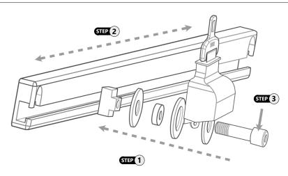
**Step 1:** Take the seat belt receiver and one of the included hardware packages. Remove the M8 screw from the package and thread the other components on it in the following order: 5/16" washer, seat belt receiver, M12 washer, spacer, 5/16" washer and the M8 T-nut. **Note:** The M12 washer has a larger hole to allow the spacer to slide inside of it.
